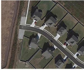
Example of a "hammerhead" turnaround at dead end
