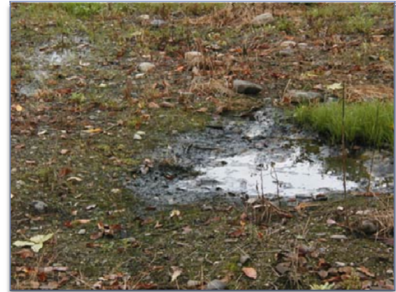
Septic System Failure Typical of the Area
